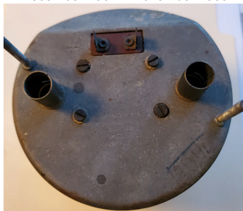
FIGURE F.1: Early pattern meter mountings vs later pattern. Note that dates provided with the above photos are best estimates and should be reasonably close, determined from vehicle production dates.
