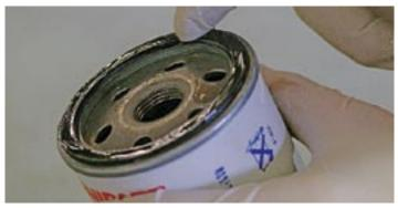
9. Before you fit the new filter apply a thin film of new engine oil around the rubber seal. You can then fit it back on the car, taking care not to damage the thread. The filter will only need to be hand tightened.
