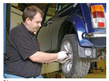
21. Now to the back where there's a little more work to do. Remove the road wheel and then the brake drum. Make sure the handbrake is off and then remove the screw securing the drum to the hub.
