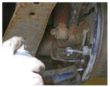
29. A can of white spray grease is a handy addition to your tool kit and this should be applied to all the linkages on the handbrake cable. Give them a quick clean with a wire brush before spraying.
