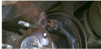
26. To prevent the brakes from squealing, apply some more copper grease to the backplate where the shoes rub and also to the face of the adjuster and the brake cylinder. You can then reassemble everything.
