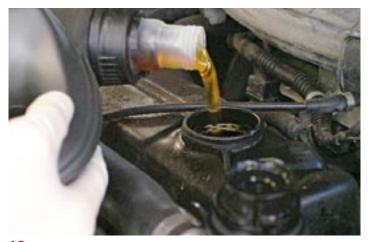
12. Once the oil has drained fully, replace the drain plug and new copper washer and fill the engine with new oil. The capacity of the Mini engine is just under 5-litres and you should use good quality 10W-40 oil.
