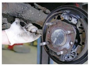
23. Inspect the handbrake cable then check that it's free to move by pulling on it. You should be able to see the handbrake mechanism move on the backplate of the hub, pushing the brake shoes outwards.
