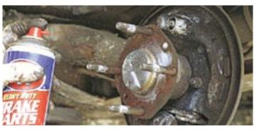
${f 24.}$  Remove the brake shoes and two springs from the backplate and then give everything a good dose of brake cleaner. Do the same with the shoes themselves and inspect the linings for excessive wear. Replace if necessary.
