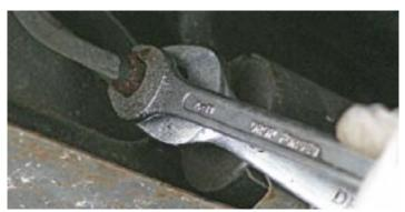
8. Disconnect the unions at either end then exchange the old filter for the new one, ensuring that the arrow's pointing in the direction of the flow of fuel. Fit it all back on the car. Make sure the unions are all done up securely and once the car's running again check for leaks.
