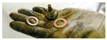
5. The sump plug also uses a copper washer to help seal against oil leaks, so this should also be replaced. Most Mini specialists should stock these along with high-street motor factors.
