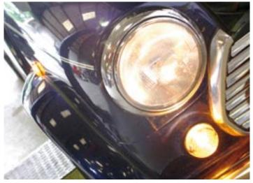
**32.** At the front, check the sidelights and indicators as well as the headlights. These are checked for alignment at your annual MoT but it's worth checking that both the dip and main beam are working correctly.
