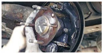
25. Use a rag to clean the backplate and surrounding areas and do the same to the brake drum itself. Don't use an air hose or similar to blow the dust away. A can of brake cleaner is relatively cheap and far healthier.
