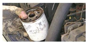
8. As well as draining the oil, you'll also need to change the oil filter. This is located on the front of the engine block and simply unscrews. Take care, as it will still be full of hot oil, so make sure the drip tray is placed underneath.
