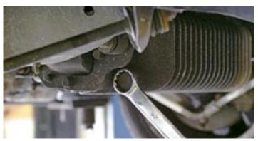
2. On a Mini, the engine and gearbox are connected so there's just one drain plug for both. Place a suitable container beneath the drain plug before removing it.
