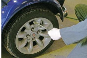
33. Finally, check the condition of the tyres and the individual tyre pressures. Before driving off go round the car and check that you haven't forgotten anything. I've heard numerous stories of people driving their cars after carrying out a service without any oil in the engine!
