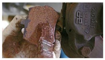
**20.** After cleaning the pads, give them a liberal coat of copper grease along the back face and the edges, but not the pad itself. This will prevent the brakes from squealing. If the pads or disc are excessively worn then replace them. Always do this in pairs.
