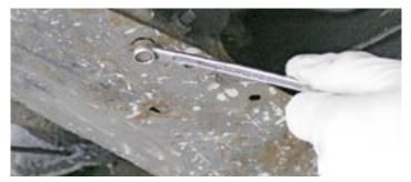
17. Two 10 mm bolts secure the filter to the subframe, so undo these first. A quick spray of WD40 or similar may help if they don't want to come out.
