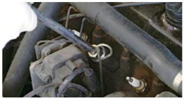
10. Spark plugs are next, although while you're removing them you should also inspect the plug leads. Any sign of damage, replace them. Clean around the plugs before removing them to prevent dirt from falling into the combustion chamber.
