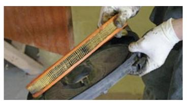
7. Undo the screws securing it to the fuel-injection system, then open the clips to reveal the filter itself. Chuck the old one in the bin and replace with a new element before fitting it back onto the car.
