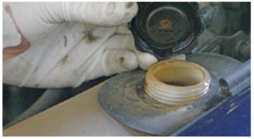
13. If the engine's cooled down enough you can also check the water level. The late-model injection Minis use a separate header tank. If yours needs fluid, then use a good quality antifreeze mix and top up to the specified level.
