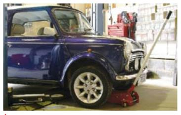
First thing to do is drive round the block a few times to warm up the oil, then park and jack the car up and place it on axle stands. This will allow access to the wheels and to the sump for draining the oil.
