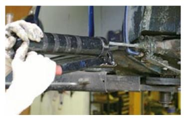
28. It's important that you keep your Mini well greased. If any of the joints are allowed to run dry then they'll wear very quickly. At the rear, apply grease from a suitable dispenser to the rear radius arm pivots.
