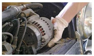
4. Also check the fanbelt, both for the correct tension and for its overall condition. If it's starting to split then it's best to change it now while the car is off the road rather than next time you are flying down the motorway!
