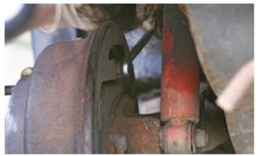
27. With the brake drum refitted, the brake shoes will need adjusting. Turn the adjuster clockwise to lock the brake drum and then turn the adjuster back until the drum will just turn freely without binding.
