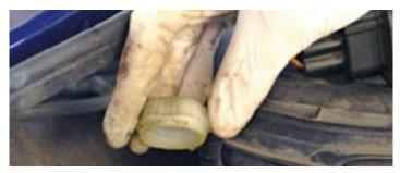
15. The clutch and brake fluid levels should also be checked and topped up with new fluid if necessary. Don't be tempted to use that old jar of brake fluid that's been sat in the shed for years either and take care not to spill any as it will remove paint with ease!
