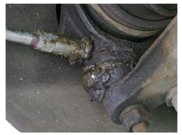
30. At the front do the same to the upper and lower steering swivel-hub ball joints. Remember to clean the grease nipple first before fitting the grease gun, and clean away any excess grease.
