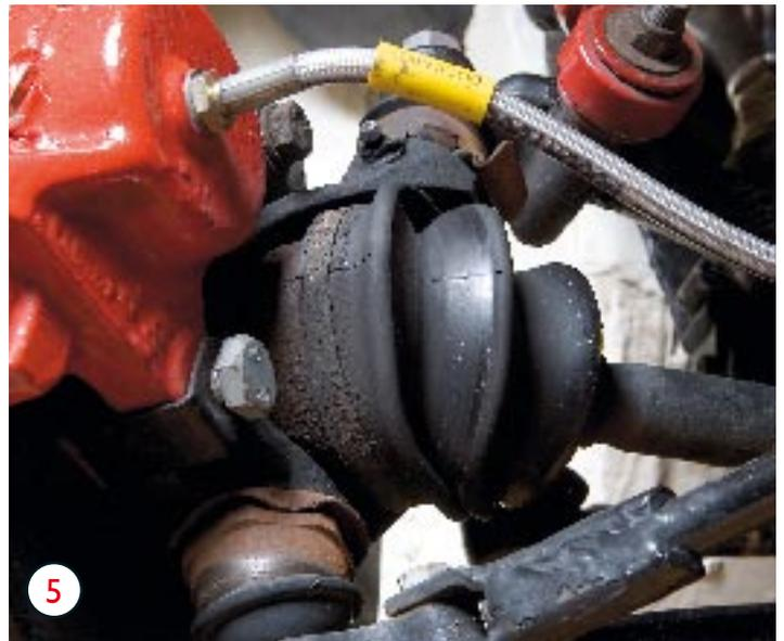
**Symptoms:** Knocking noise from the front with the steering on lock
